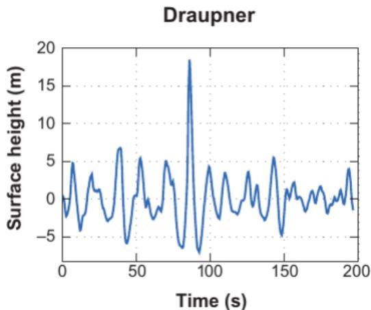
New Year wave recorded at the Draupner platform in the North Sea on January 1, 1995. The crest height is  $\approx$  18.5 m and exceeds the Significant Wave Height of 11.8 m by a factor of 1.54.
