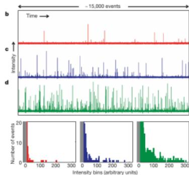
The supercontinuum radiation used is generated by sending picosecond seed pulses at 1,064 nm through a highly nonlinear microstructured optical fibre with matched zero-dispersion wavelength. The output is red-pass filtered at 1,450 nm and stretched so that many thousands of events can be captured with high resolution in a single-shot measurement.
