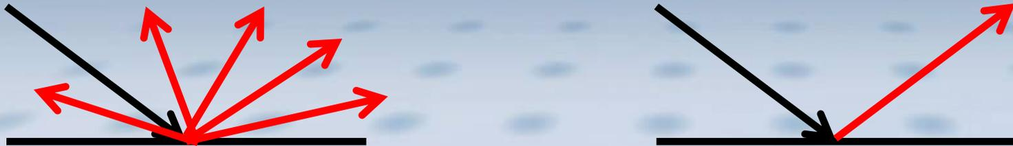
Thermal conductivity (limited by size effect) of silicon is larger when fiber surface is polished .
