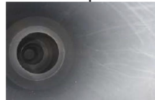
Black coating on inner surface and baffles
